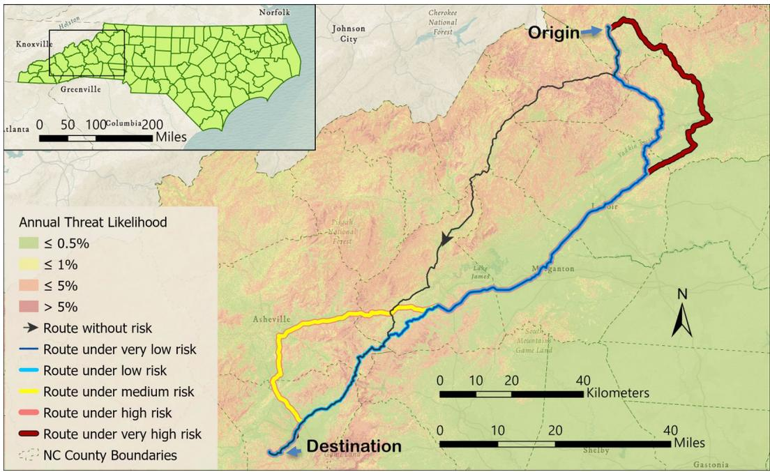
Figure 3.15. Map of shortest paths of a single origin-destination pair under different scenarios of landslide risks.
