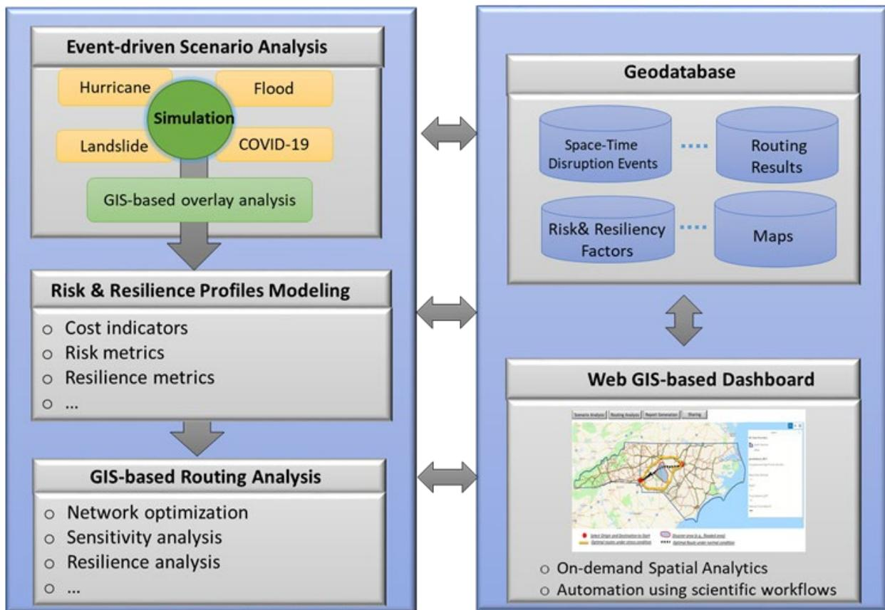
Figure 1.1. Design of the Geo-FRIT framework for risk-based freight routing analytics (Geo-FRIT: a web-based geospatial analytics tool for quantifying freight risk and resilience in transportation).
