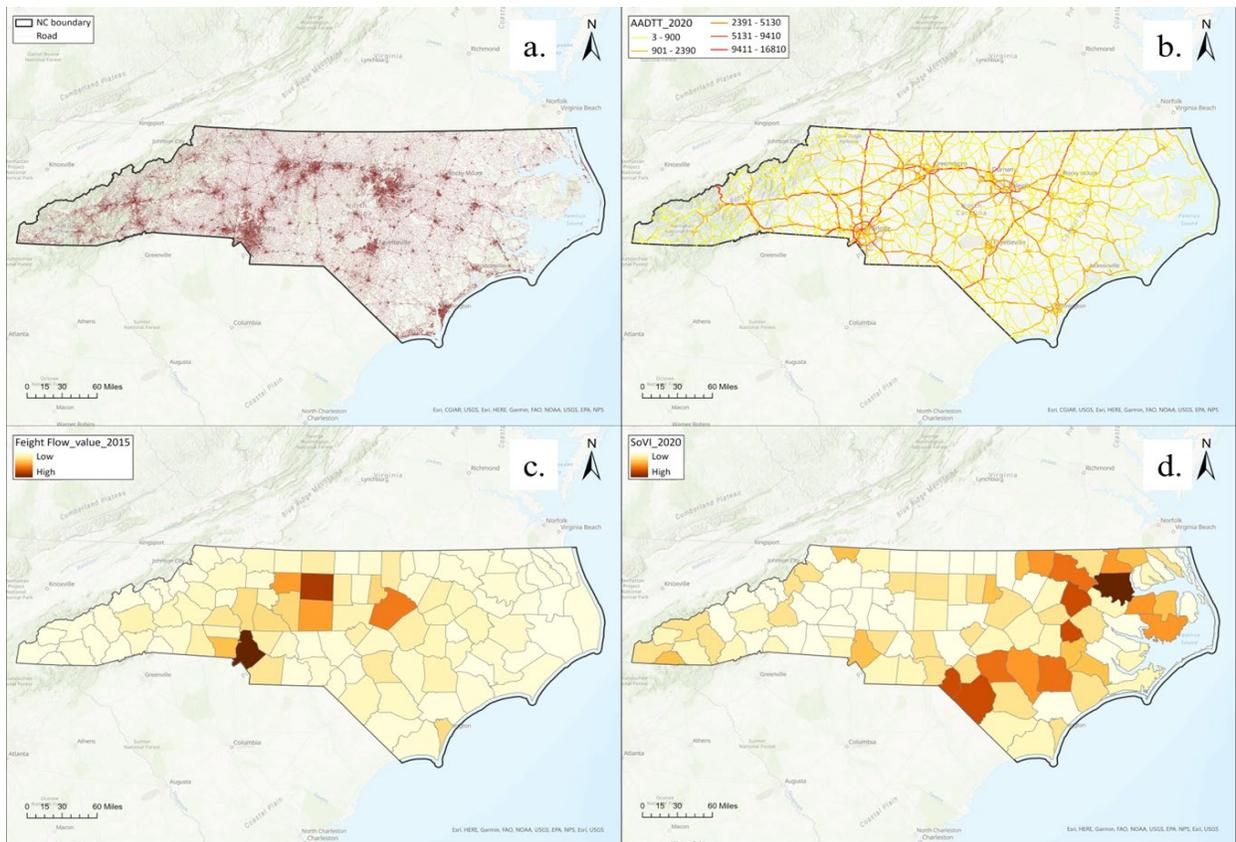
Figure 3.10. Maps of factors for criticality estimation (a. Roads, b. AADT, c. Freight flow value per ton, and d. SoVI).
