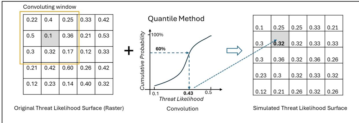
Figure 3.13. Illustration on the convolution-based spatial simulation approach for representing the threat likelihood of an extreme event in different severities (60<sup>th</sup> percentile was used as an example here).
